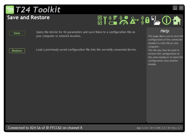
Here you can save the module settings to a file on your PC so that they can be later loaded back into the same or different module.
