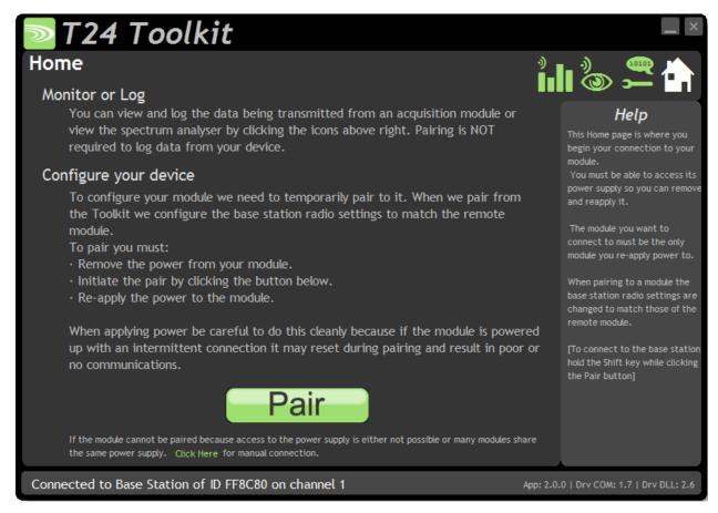
You now have successful communications with the base station so you can now pair with your remote X24 module or you can select the Spectrum Analyser mode or Data Provider Monitor mode.
